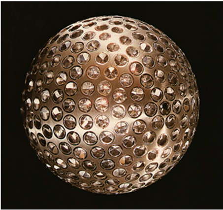
Figure 2. LAGEOS, made specifically for SLR [Wikipedia: LAGEOS].
