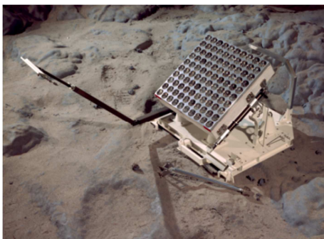
Figure 1. Laser Retroreflector "Apollo 11" (Science Museum).
