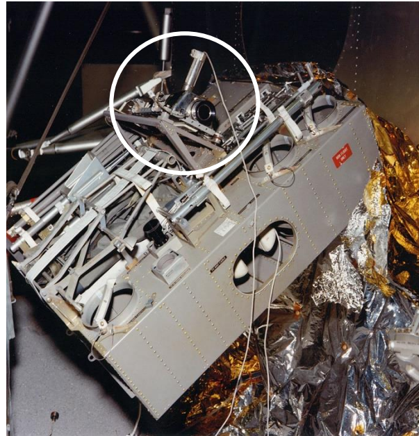
The TV camera is mounted on the MESA (Modular Equipment Storage Assembly) with a tilt, so that also the bottom of the ladder would be visible on the diagonal of the image.
